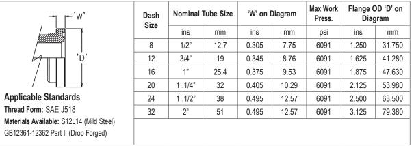
NOTE: Komatsu use flanges that comply with Code 61 and Code 62 in all respects except O-Ring groove dimensions. Refer to PIRTEK fittings catalog Section B for details. They comply to a JIS Standard, and include a Dash 10 size.
