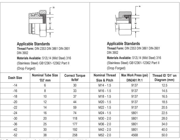
Note: The torque values given are for plated carbon steel components without lubrication.
